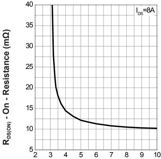
V<sub>GS</sub> - Gate - Source Voltage (V)
