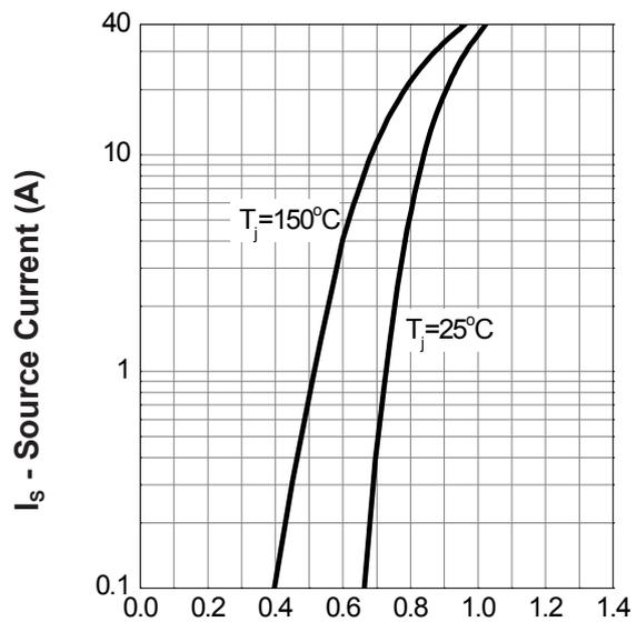
V<sub>SD</sub> - Source - Drain Voltage (V)
